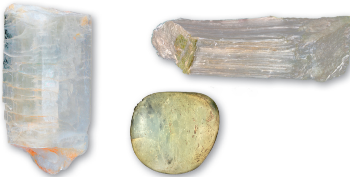
Tremolite, from mineral to rock: single crystal (left); easily detachable and flexible fibrous crystals of white asbestos (top); and compact (tenacious) pebble of microcrystalline tremolite, known as tremolitite or nephrite (bottom).
